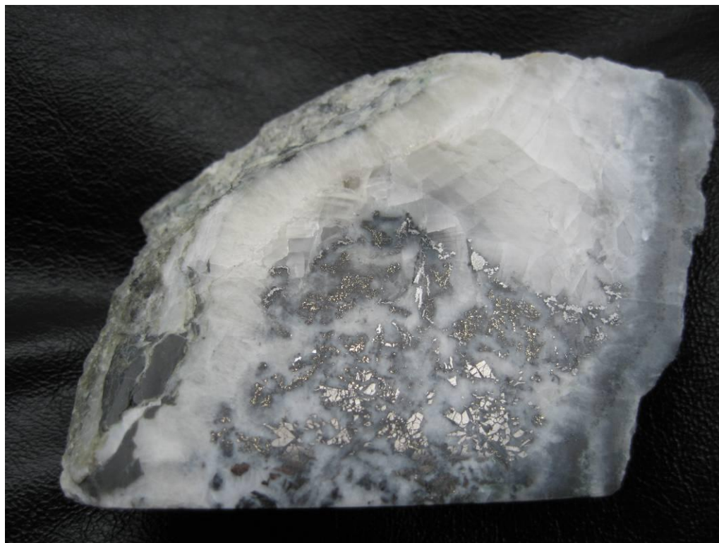
[B] Detail of [A] showing part of intersection (344.1 g/t Au over 0.35 m; red section in [A] above) where coarser-grained arsenopyrite and electrum needles are associated with, and contained within roscoelite. Core width 63 mm (Source: BCGold)
