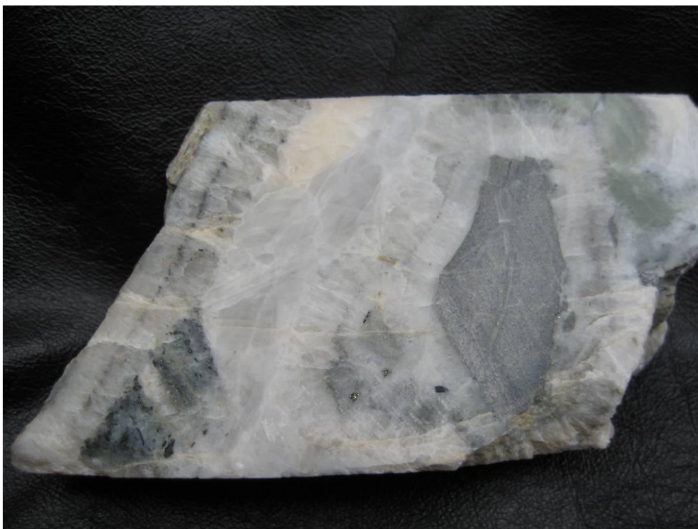
[B] Detail of [A] showing part of the vein intersection (30.7 g/t Au over 0.41 m; blue section in [A] above) where electrum and associated fine roscoelite occur both within and without ~1 cm thick overgrowths of cockscomb quartz on vein margin (left) and breccia clast of quartz-sericite altered argillite. Core width 63 mm (Source: BCGold)
