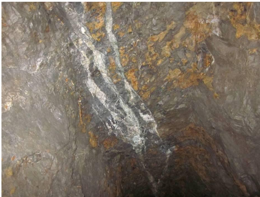
[B] Horsetail quartz veining on 5 Level. Individual vein widths approximately 1 cm to 10 cm (Source: Snowden, 2011)
