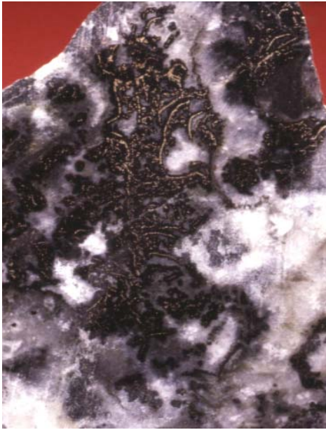
Figure 10. Bright electrum in dark roscoelite, 8 cm across. U.B.C. specimen #6724; Mark Mauthner photo.
