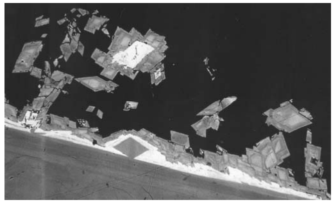
Figure 8. Arsenopyrite crystals (gray) with löllingite (white) in polished section back-scatter electron image 250 µm across, by M. Raudsepp. U.B.C. collection.
