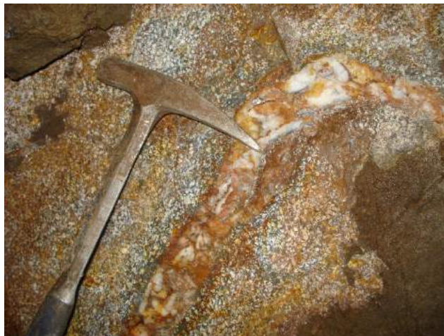
FIGURE 8 ENGINEER VEIN DIMINISHES TO 10 CM WIDTH WHEN HOSTED IN FELDSPAR PORPHYRY DYKE. IMAGE FROM 401-6 RAISE ON 4 LEVEL (D. O'BRIEN, 2011).
