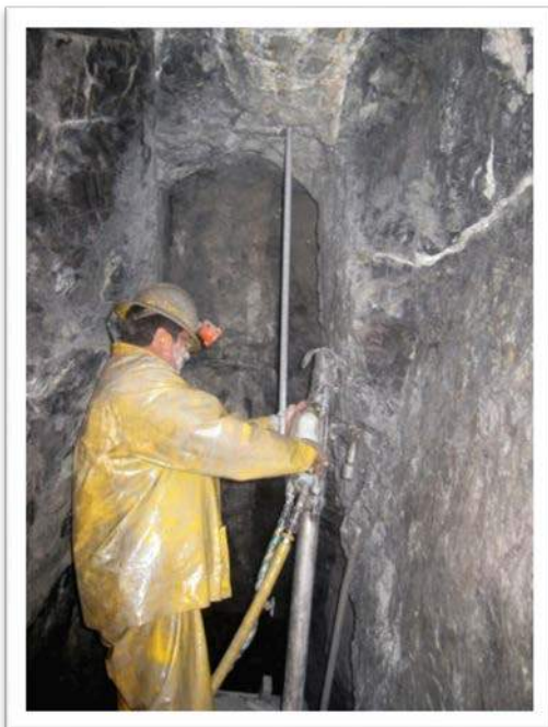
FIGURE 41 PREPARING TO BLAST BULK SAMPLE 505-5 OF THE ENGINEER VEIN FROM 5 LEVEL
