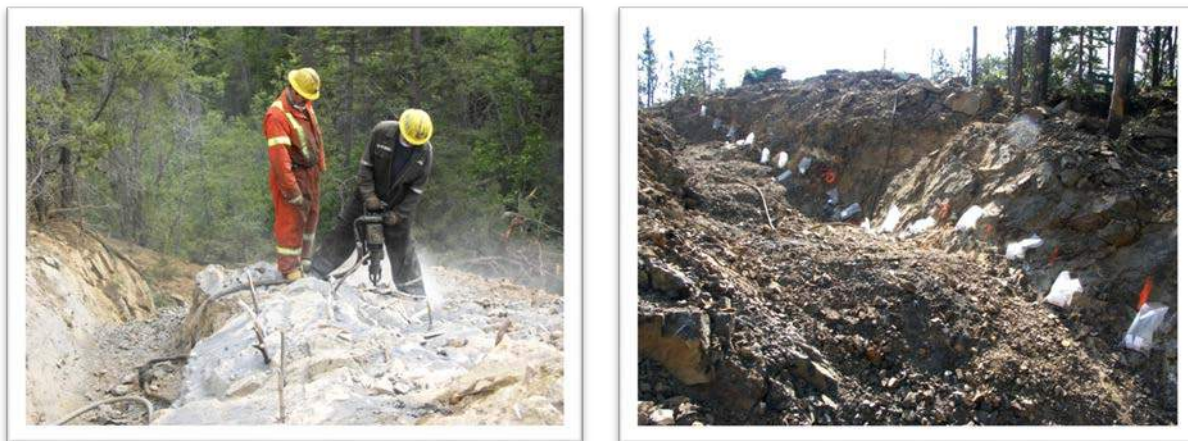
FIGURE 36 DOUBLE DECKER VEIN - BLASTING AND CHANNEL SAMPLES
