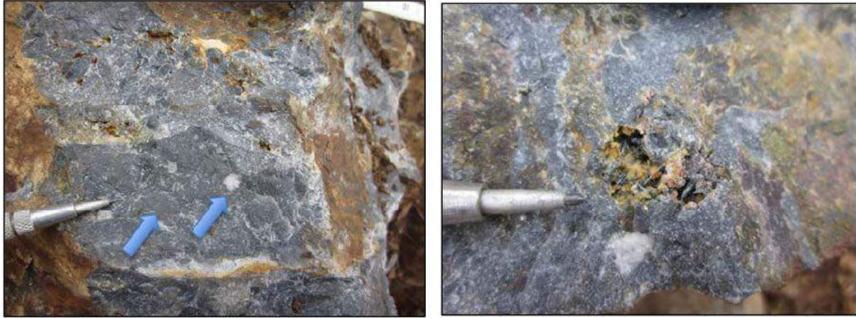
FIGURE 14 SHEAR B 'STAGE 1' HYDROTHERMAL BRECCIA. BLUE ARROWS POINT TO SULPHIDE AND QUARTZ CLASTS WITHIN A FINE-GRAINED QUARTZ-SULPHIDE MATRIX. STIBNITE CRYSTALS LINE OPEN SPACE VUGS. (DEVINE, 2011)
