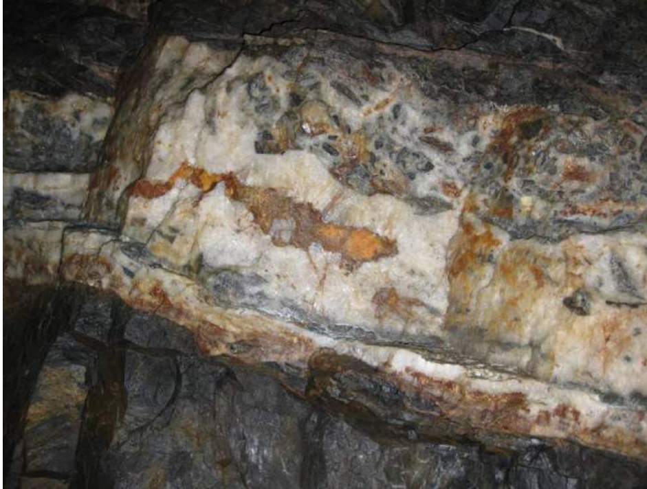
FIGURE 12 DOUBLE DECKER VEIN ON 5 LEVEL. MULTI-STAGE QUARTZ-CALCITE SHOWING BRECCIATION AND BANDING. WIDTH 20 CM (DEVINE, 2008)
