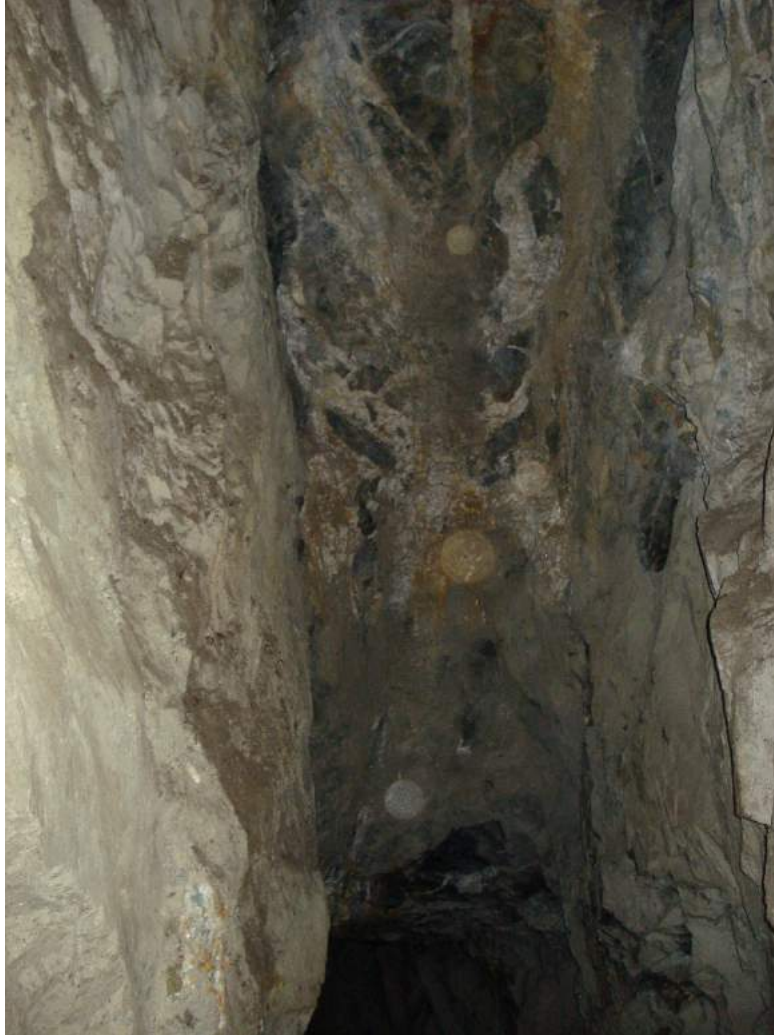
FIGURE 7 ENGINEER VEIN SHOOT 505-3 (NE FACE) ON 5 LEVEL IS OVER 2 M WIDE NEAR CONTACT WITH FELDSPAR PORPHYRY DYKE (D. O'BRIEN, 2011).
