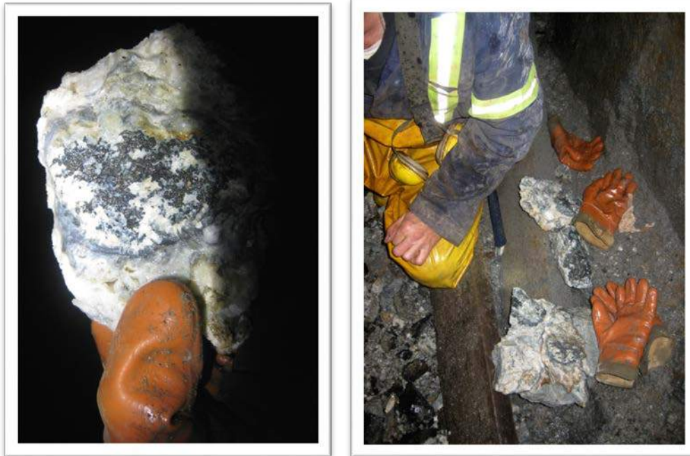
FIGURE 42 ELECTRUM / ROSCOELITE NODULES SELECTED FROM BULK SAMPLE 505-5 FROM THE ENGINEER VEIN
