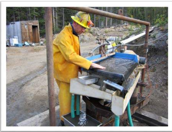
FIGURE 67 FINISHING DEISTER TABLE
