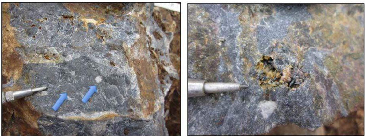
FIGURE 31 STAGE 1 HYDROTHERMAL BRECCIA AND SILICIFICATION ALONG SHEAR B (DEVINE 2011). SULPHIDE AND QUARTZ CLASTS WITHIN A QUARTZ-SULPHIDE MATRIX. STIBNITE CRYSTAL LINE OPEN SPACE VUGS.
